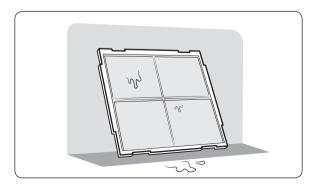
Clean the air filter with a vacuum cleaner or soft brush. If dust is too heavy, then rinse it with running water and dry it in a ventilated area.
