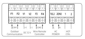
The output of hot coil terminal is AC 220 V / 230 V (The same as Indoor Unit's input Power)
