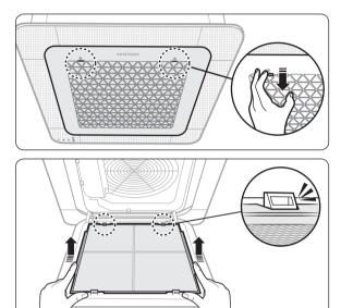
Push down the hooks at each side of the front grille to open the grille.
