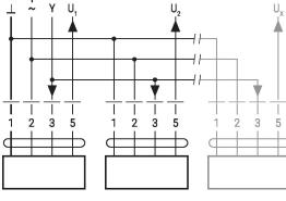
• Max. 8 actuators in parallel • Parallel operation is permitted only on non-connected axes • Do not fail to observe performance data with parallel operation
