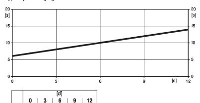
[d] = Power failure in days [s] = Pre-charging time in seconds
