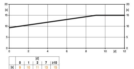
[d] = Power failure in days [s] = Pre-charging time in seconds PF[s] = Bridging time
