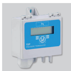
TDP-S/TDP-D/TDP-PI Pressure sensor. Enables you to control the pressure in the fan inlet. Pressure range: 0-2500 Pa. Output signal: 0-10V/4-20 mA.
