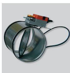
REMP Motorised damper, opens proportionately and is controlled by the BEAS control module. Power supply: 24 VAC or 24 VD, depending on the models.
