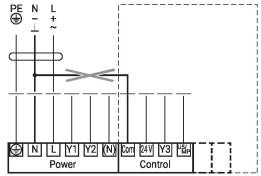
Power supply must not be connected to the signal terminals!
