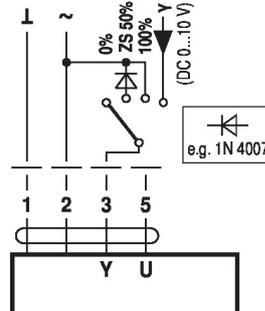
Control remotely 0...100% with positioner SG..
